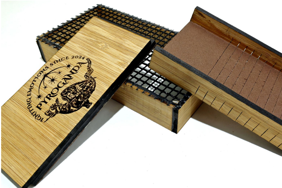
Figure 41: In this image, on the left, you can see the cover plate made from two cut-out elements that were glued slightly offset against each other. This results in one plate slightly protruding from the saw guide, making it easier to open (see also figure 40 on the left). Alternatively, one plate can be made slightly larger. In any case, two plates need to be glued together to achieve the necessary thickness for applying pressure to the sticks. In the center, the matching sieve is visible, made from slightly longer sides onto which a non-stick grill grate has been glued. On the right, you can see the glued foam rubber layer that has been sawed through together with the bamboo sheet.
