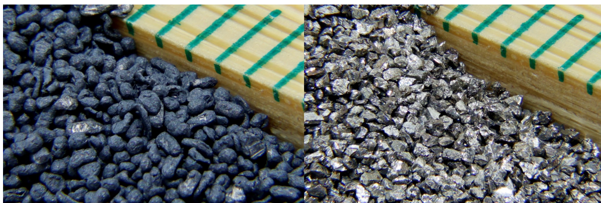
Figure 2: Macro photograph of two high-performing metal types. Left: magnesium (300–600 \mu\text{m} , <50 mesh); right: magnalium 50/50 (200–400 \mu\text{m} , >60 mesh). Scale divisions represent 1 mm.
