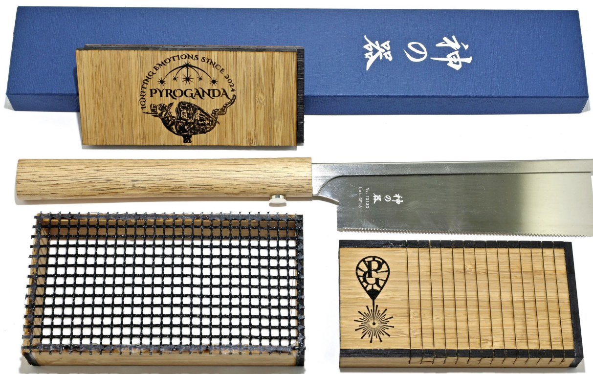
Figure 4: Custom-made sawing guide and Japanese 'Dozuki'-type pull saw
