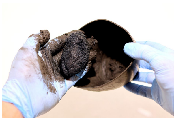
Figure 6: The paste is then kneaded by hand. After hydration of the CMC, a well-processable paste is obtained.
