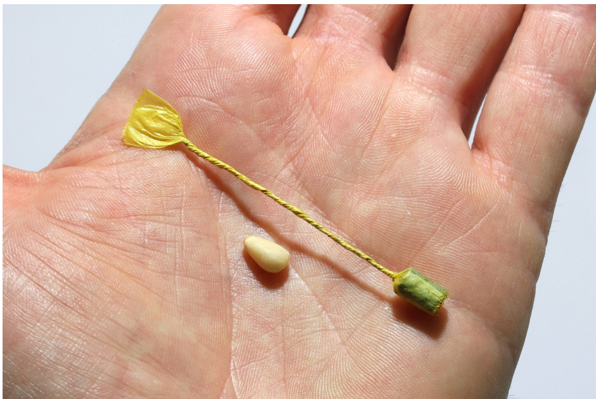
Figure 26: A finished Dragon Tear. The pine nut next to it weighs exactly the same (112 mg). Even Dragon Tears weighing less than 100 mg can still amaze with their impressive spark display.
