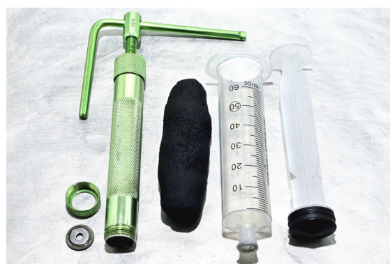
Figure 7: The paste can be extruded from a syringe with moderate force. However, a clay extruder with a screw mechanism provides easier handling.
