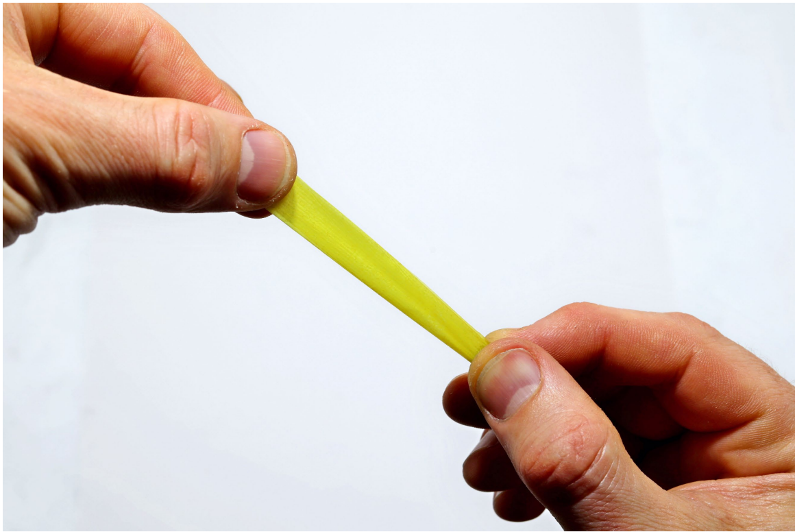
Figure 21: During the rolling, the sparkler is kept facing upwards so that the metal remains in contact with the pellet.
