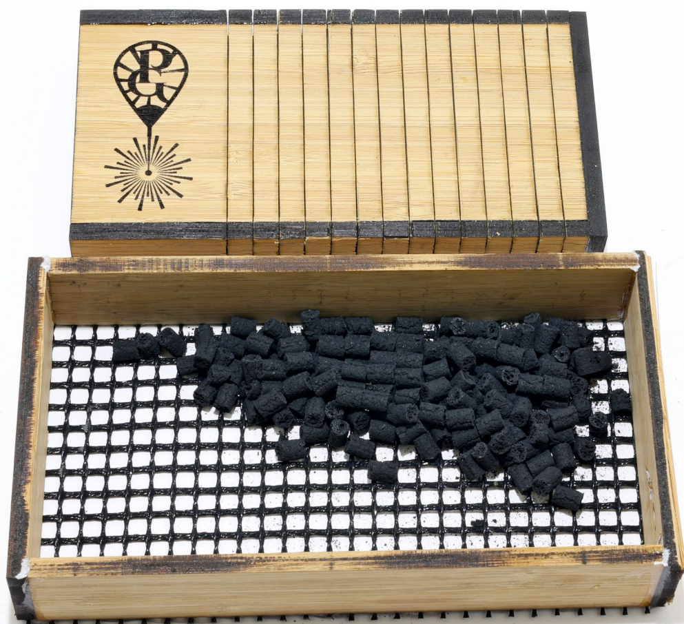
Figure 14: An adapted coarse sieve is used to efficiently separate the pellets from the sawdust.
