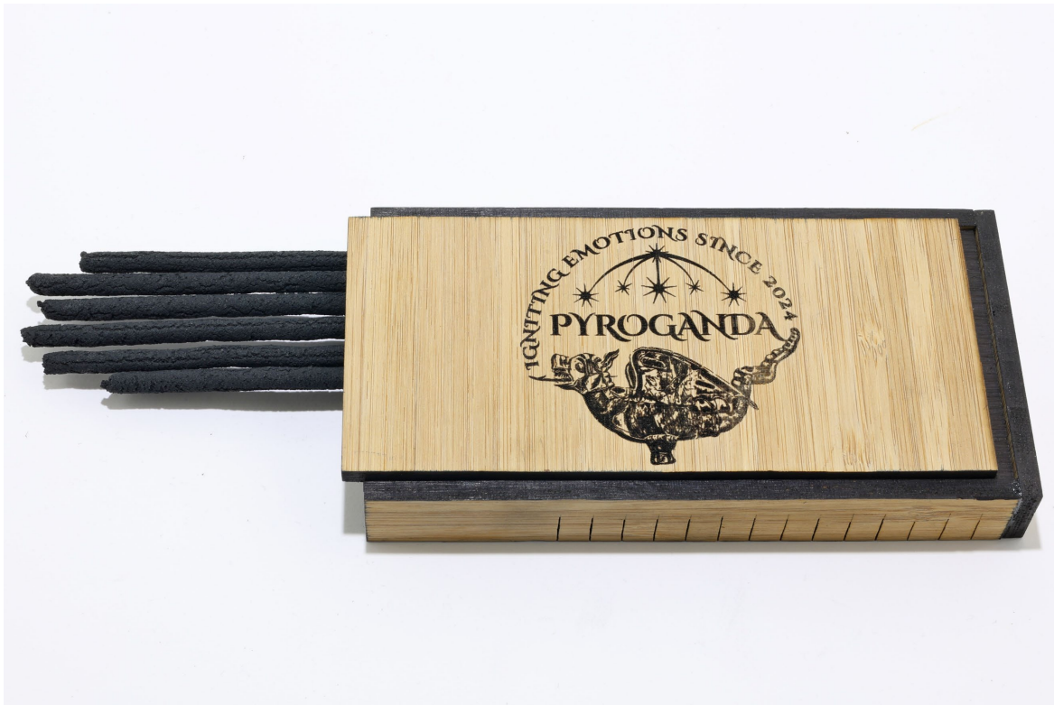
Figure 11: The lid is placed on top of the rods, and the entire assembly is inverted.
