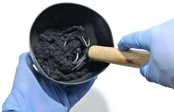
Figure 5: The composition and water are initially mixed using a Danish dough whisk
