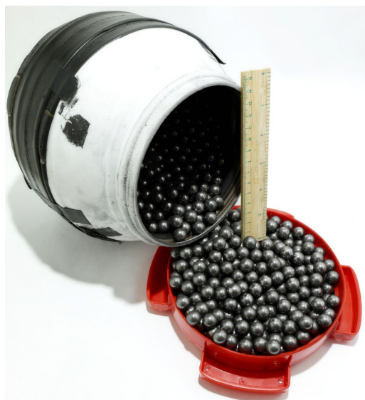
Figure 3: 3.6-liter milling jar with 12 mm steel grinding media
