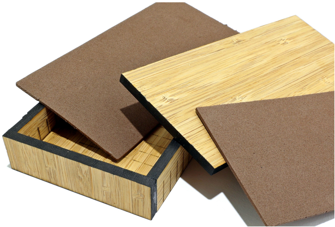
Figure 39: The components are assembled, after which thin foam mats are glued to the interior and the loose panel.
