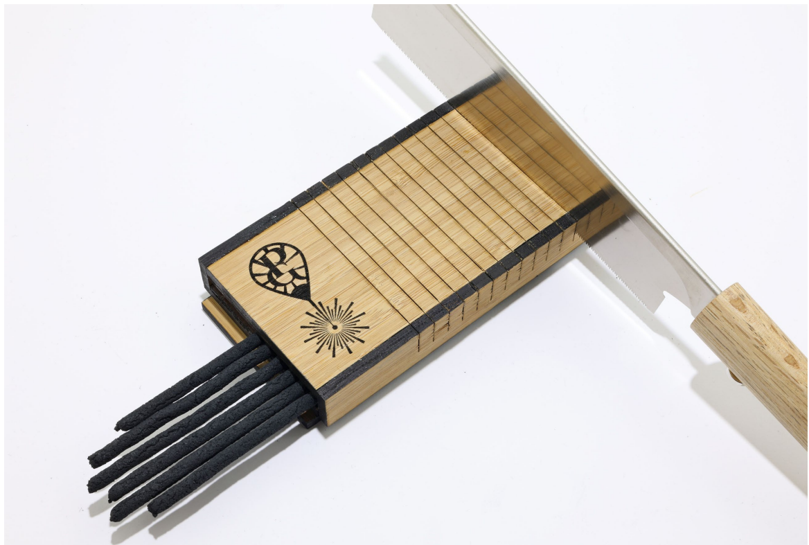
Figure 12: The rods are then cut into ~7 mm segments using the pull saw, while applying gentle pressure on the sawing guide to lock the rods in place. While Western in origin, the pellet process resonates with the spirit of Japanese tradition.
