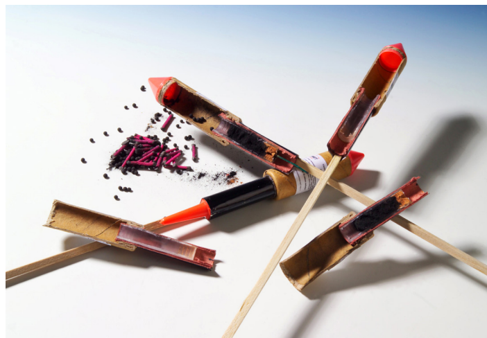
Figure 2. Dismantled fireworks rockets of category F2 (photo: BAM).
