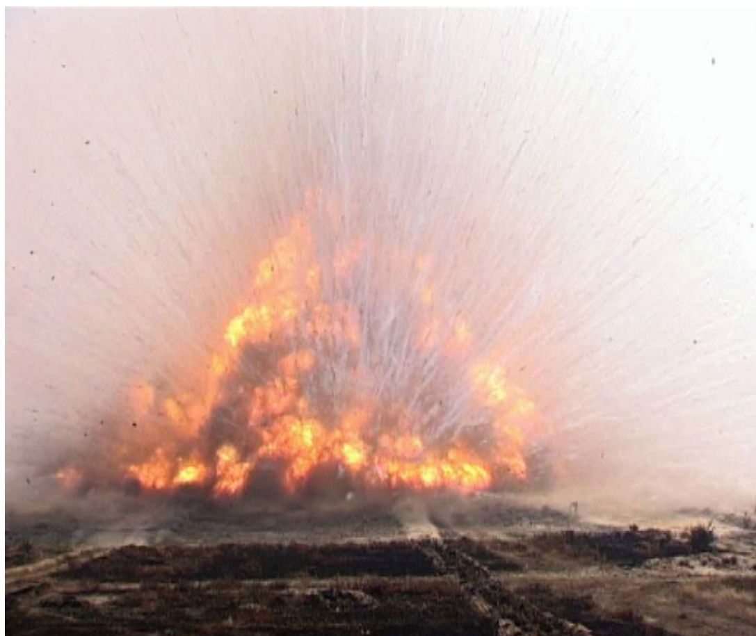
Figure 1. Full-scale ISO container testing of stickless rockets.
