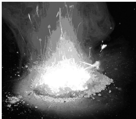
Figure 2. Combustion of bulk pyrolant.
