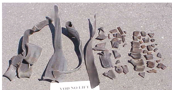
Figure 8. Test 3: report shells (booster initiated)
