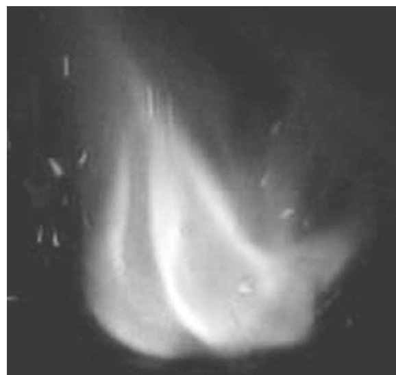
Figure 5. A photograph of a burning pellet of the lilac composition showing the brighter and lighter outer flame envelope.
