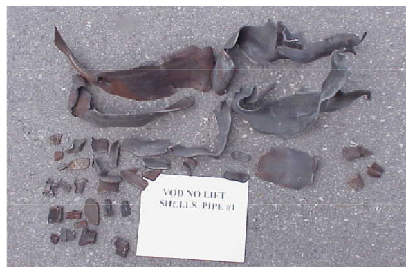
Figure 9. Test 4: report shells (15 g black powder initiated)
