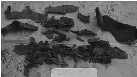
Figure 15. Test 9: Loose spherical 12 mm Ø red stars (2.6 kg)
