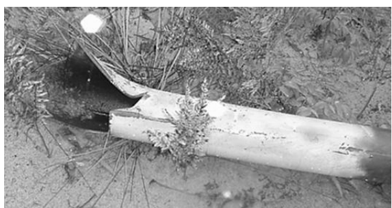
Figure 26. Detail of damage to non-initiated end of pipe in Trial 4. Note sign of incipient splitting from damaged end to right edge of photograph.
