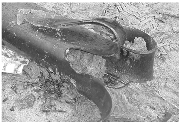
Figure 25. Damage resulting from booster and explosion of first few shells (Trial 4).
