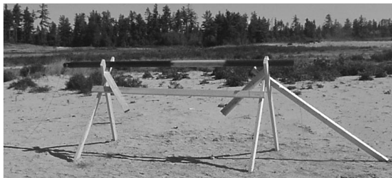
Figure 7. Assembled pipe on wooden frame (Initiation from right).
