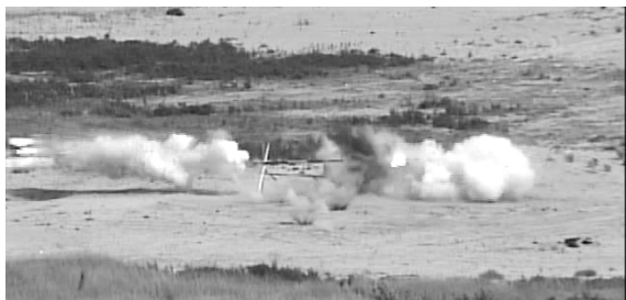
Figure 15. Shells being propelled from end of pipe in Trial 2.
