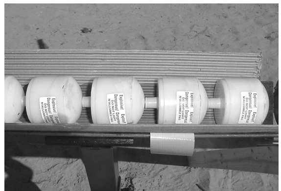
Figures 18a (left) and 18b (right). Plastic cased report shells being prepared for loading in steel pipe.
