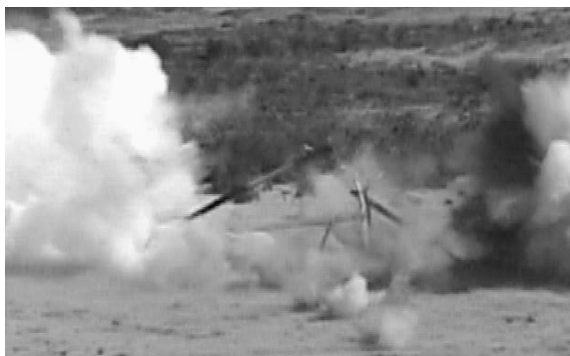
Figure 9. Fireball at opposite end and rotation of pipe.
