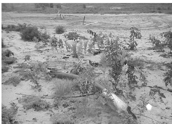
Figure 24. Length of pipe thrown from test location in the background (Trial 4).
