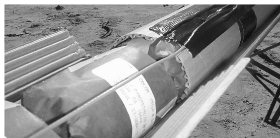
Figure 6. VoD probe taped to the side of the column of 76-mm star shells.
