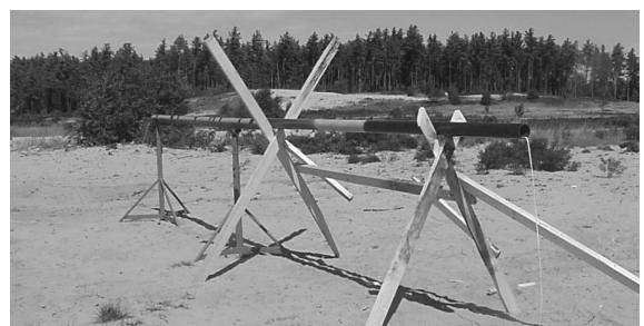
Figure 13. Assembly of 76-mm star shells ready to be pulled into pipe.
