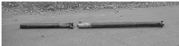
Figure 20. Damage due to booster at right end of pipe in Trial 3. Damage towards left end is at location of last shell in pipe.
