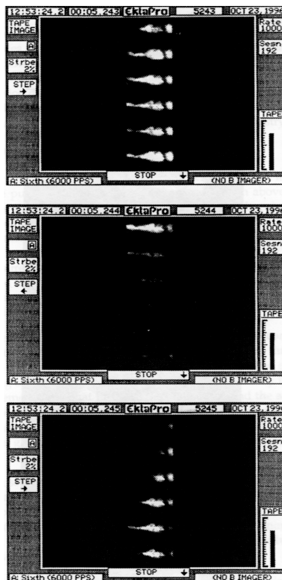
Figure 6. High-speed video record of a low frequency pyrotechnic whistle, showing the active (bright) and quiescent (dark) combustion cycles. To slow the whistle frequency to enable a full cycle to be recorded, an extended chimney tube was fitted to the device. When, in another experiment, a 'normal' 3 kHz whistle was located and ignited at a distance of 15 mm from the end of the low frequency whistle, pointing directly at the mouth of the extended tube, the combustion frequency of the first whistle was observed to increase. [1] This experiment demonstrated that the whistling frequency is controlled by the incoming pressure pulses (normally as a result of reflection from the tube mouth).
