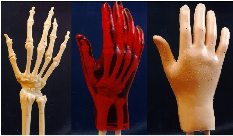
Figure 1. Construction of skeletal hand simulant in open-palm version.
