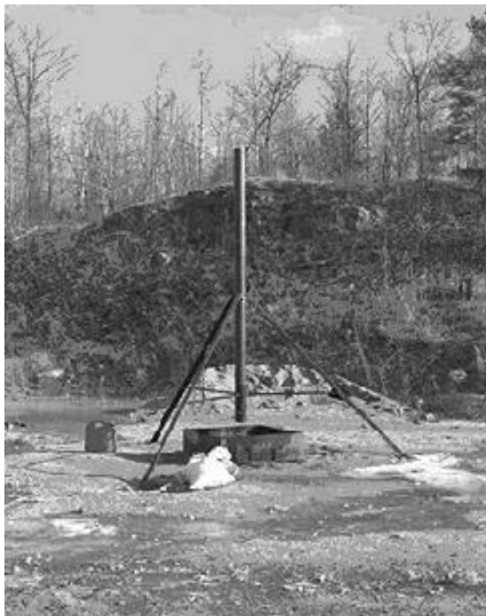
Figure 2. Height-to-Detonation test configuration.
