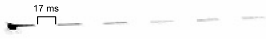
Figure 5. Composite image of a glitter dross droplet just prior to the start of the flash reaction. Note the droplet is moving from right to left.
