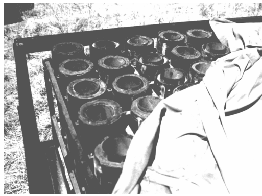
Photo 5. An example of a "dense-pack" style mortar rack containing "matrix mortars," which are "double-walled" and foamed.
