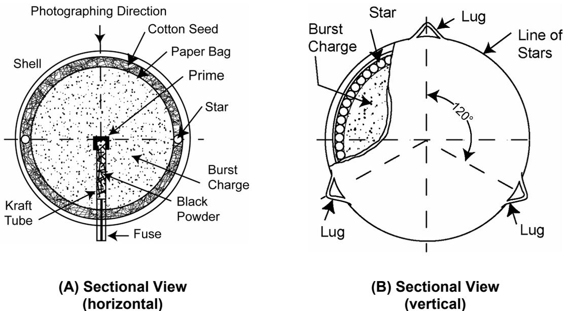
Figure 15. The construction of the sample ring shell.
