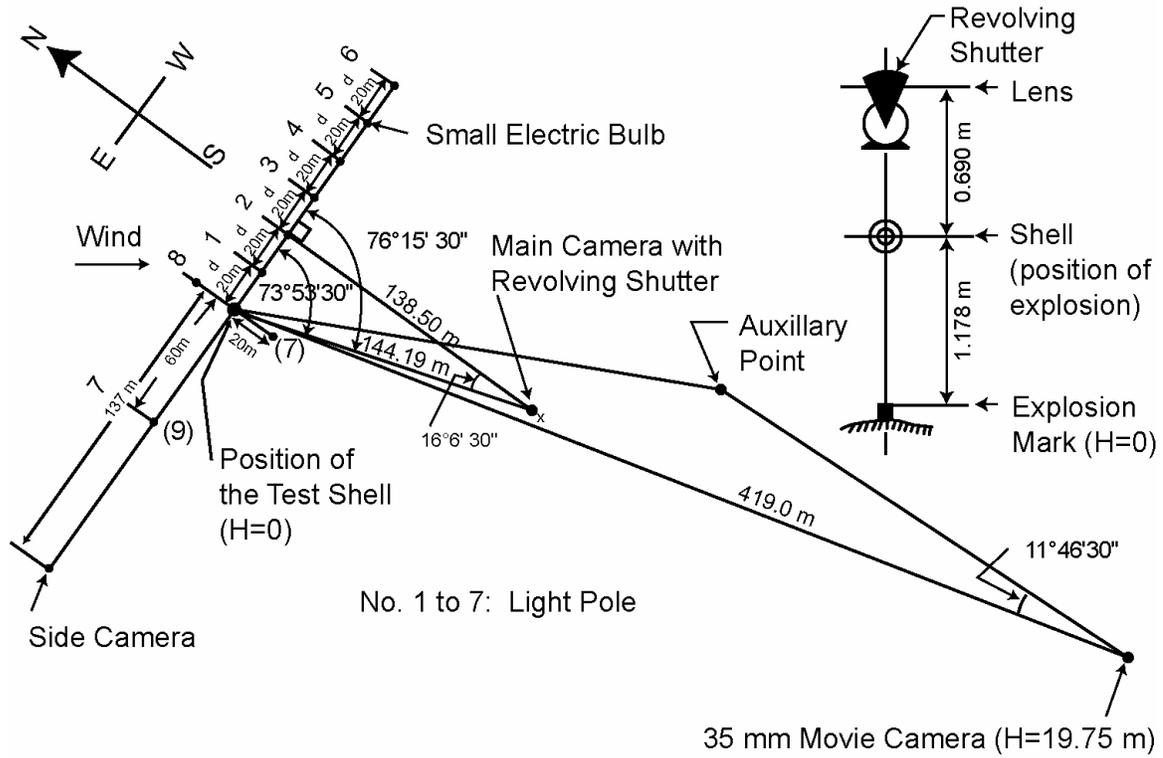
Figure 18. Arrangement of the instruments for the exploding shells.
