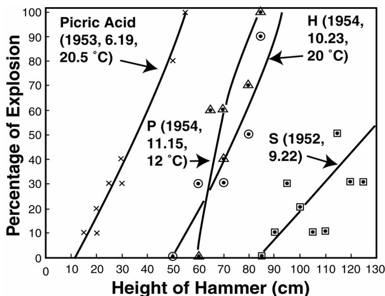
Figure 13. The results of drop hammer test of burst charges.
