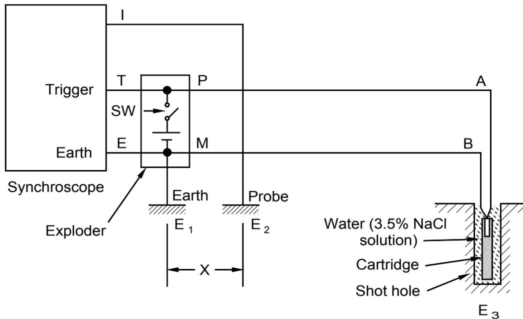
Figure 1. Circuit which produces a noise from one-hole blasting.  $I = \text{input}$ .
