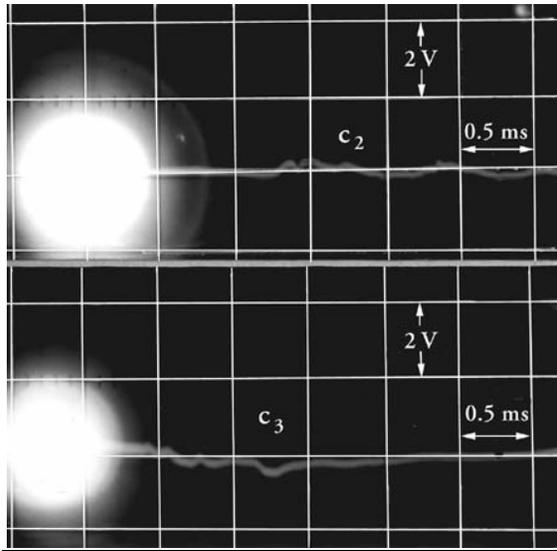
Figure 5 Noises from an explosive charge in a short cartridge (diameter: 35 mm, length: 220 mm, charge: 177–190 g, detonation velocity: 1,400 m/s),  $c_2$ : noise from a charge without electric initiation;  $c_3$ : noise from a charge with electric initiation, which is independent of the measuring circuit.
