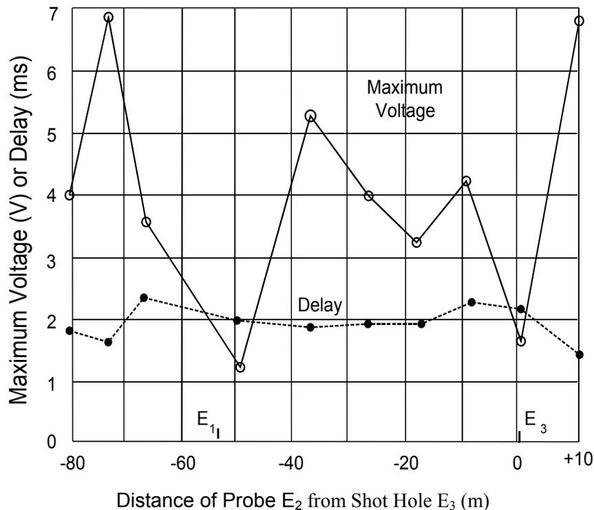
Figure 6. Influence of the position of the probe  $E_2$  to the shot hole  $E_3$  and to the ground of the exploder  $E_1$  on the voltage of a noise. (Delay times from switching on to the initiation of a detonator are also shown.)
