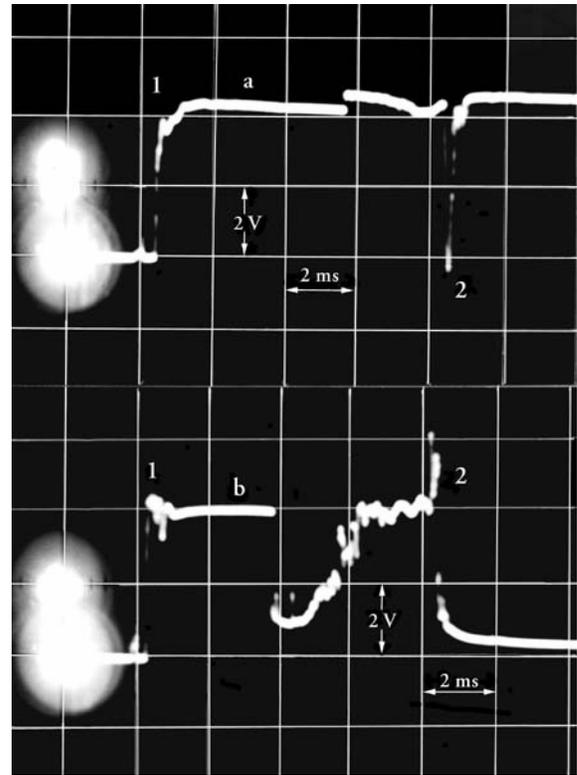
Figure 11. Noises from a double-hole blasting: *a* and *b* correspond to those in Figure 10 respectively. 1: from a detonator; 2: from a small cartridge which explodes with a delay.
