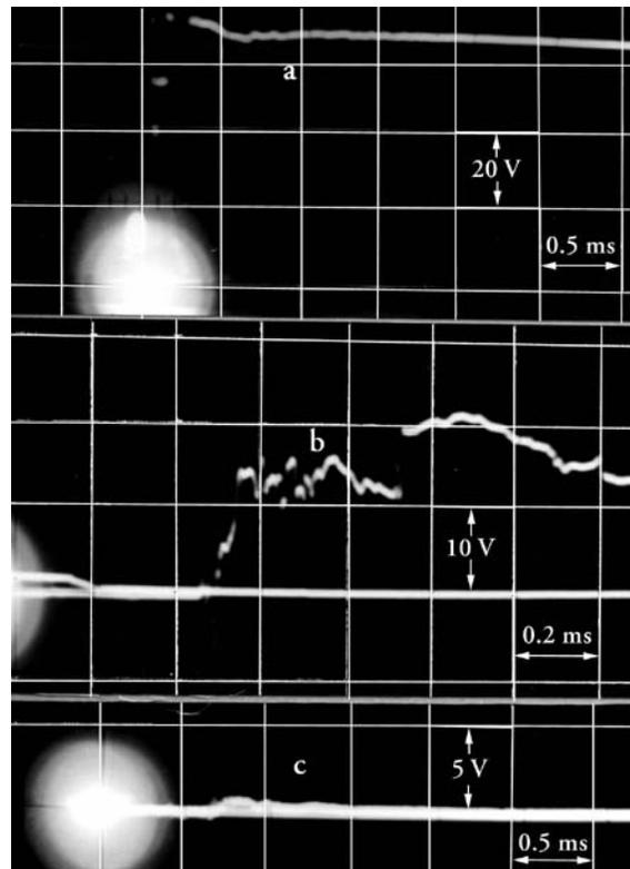
Figure 4. Noise from an explosive charge in a long cartridge (diameter: 35 mm, length: 440 mm, charge: 315–386 g, detonation velocity: 1400 m/s), a: blasting voltage; b: noise from a charge; c: noise from a charge under disconnection of blasting circuit.
