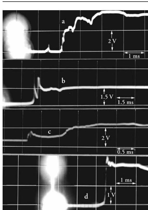
Figure 7. Noises from a detonator, blasting current: a = 3.3 A; and b, c, d = 1.6 A.
