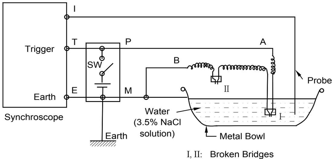
Figure 9. Circuit for imitation test of noises from double-hole blasting in a room.  $I$  = input,  $SW$  = switch in exploder.
