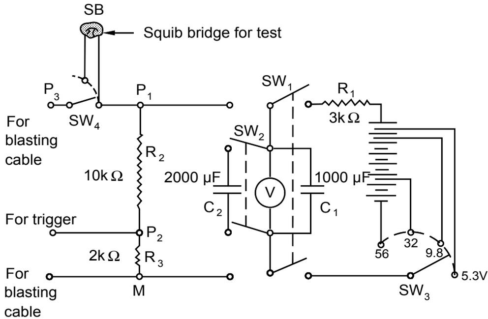
Figure 2. Circuit of exploder.
