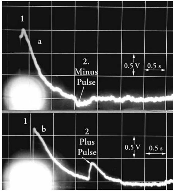
Figure 10. Noises from an imitation test, *a*: the plus terminal of the exploder is connected to the broken bridge, which is first put into the water, *b*: reverse of *a*.
