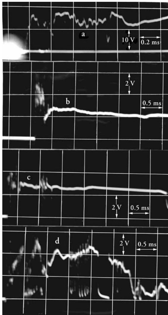
Figure 8. Noises from all explosive charge. The probe  $E_2$  and the shothole  $E_3$  are separated in the case of a, and connected, in the case of b, c, and d (long cartridges, see Figures 4 and 5).
