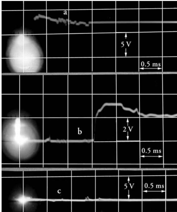
Figure 3. Noises from a detonator, a: blasting voltage for b; b: noise from a detonator; c: noise from a detonator under disconnection of blasting circuit.
