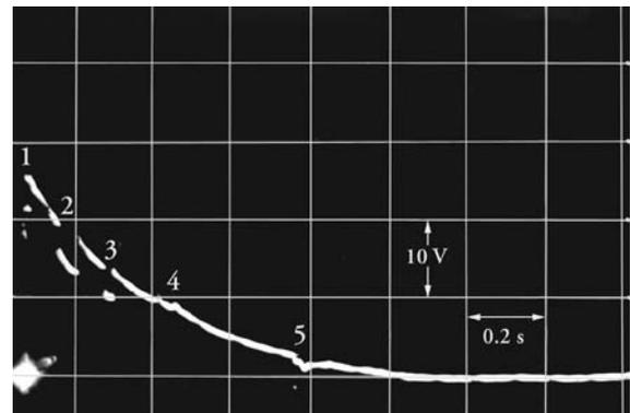
Figure 12. Noise from a five-step delay blasting using delay detonators.
