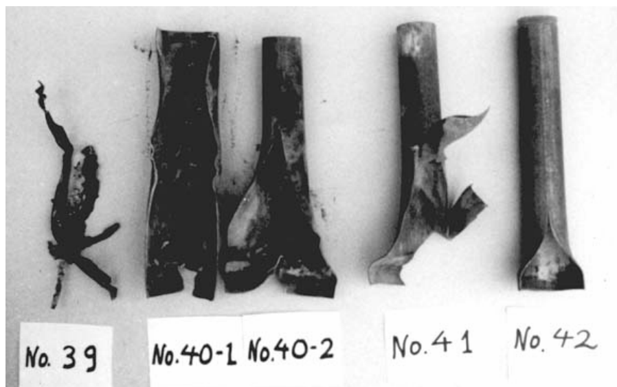
Figure 8. The debris obtained after the iron tube test.
