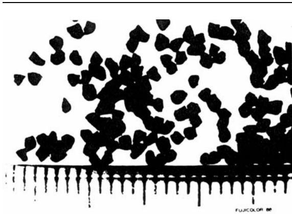
Figure 1. Configurations of Black Powder grains between two sieve openings 0.850 mm and 1.000 mm. The scale is in mm. (Table 1. No. 8)
