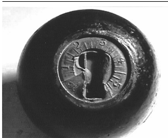
Figure 3. A photo of a Bormann fuse in place on a 6-pounder cannon ball.
