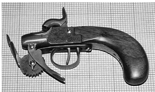
Figure 1. Photo of Eprouvette, [9] an early Black Powder Tester.
