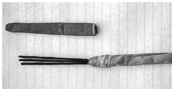
Figure 1. Photo of a shell leader containing the new fast burning black match. (Note that the three exposed fuses have been separated slightly for clarity.)
