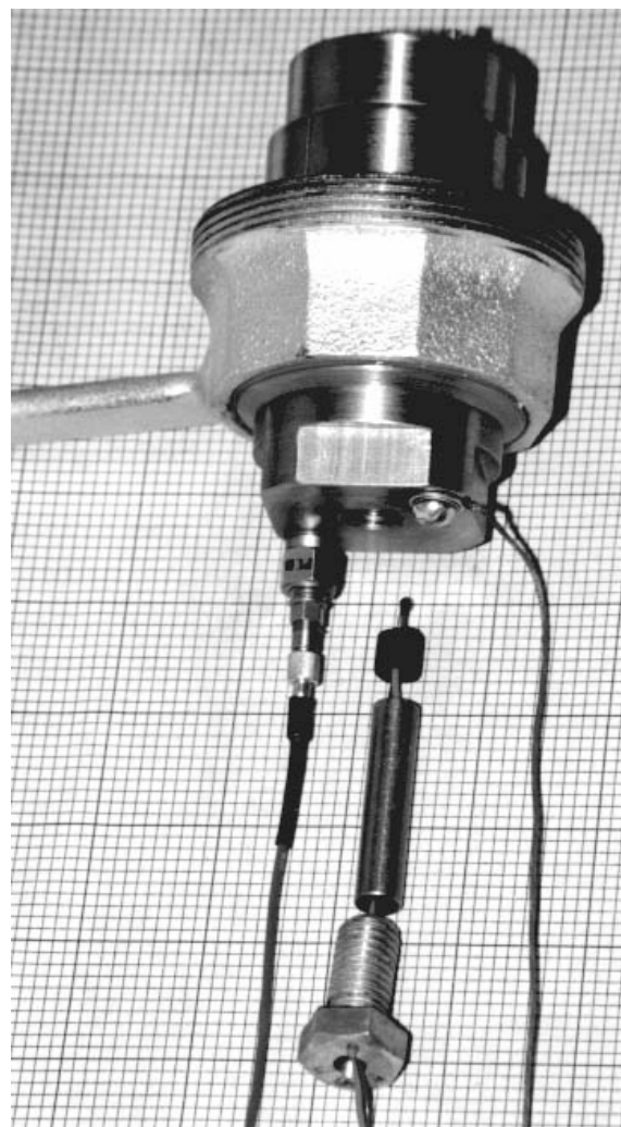
Figure 5. Breech plug for mortar portion of test instrument.
