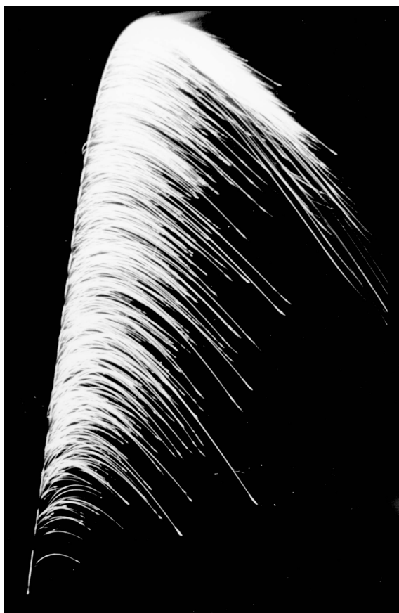
Figure 2. A Black Powder comet with 10% flake titanium (10–20 mesh).
