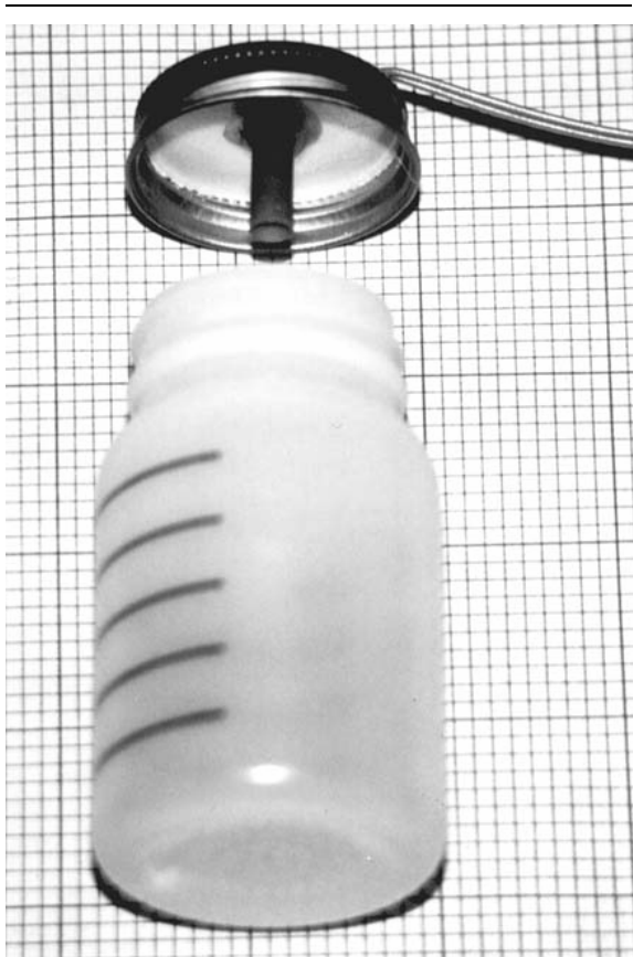
Figure 4. An electric match installed in the cap of a test salute casing (polyethylene bottle).
