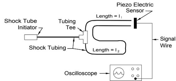
Figure 5. Determination of shock velocity within shock tube.
