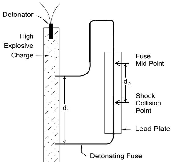
Figure 2. Dautriche method for measuring detonation velocity.
