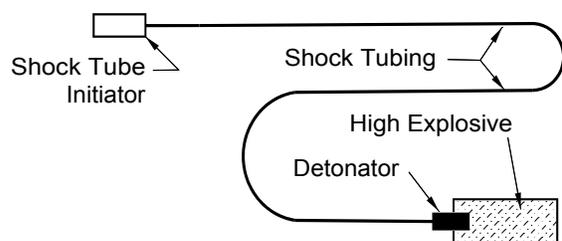
Figure 1. Shock tube initiation system for high explosives.
