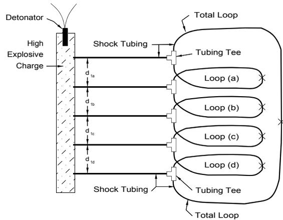
Figure 3. Shock tube method for measuring propagation velocity.
