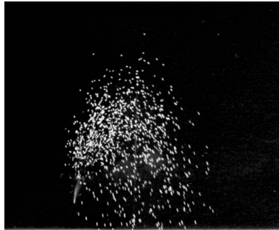
Photo 8. Fountain test, 10–20 mesh Pyro-Flake (90-6-4).
