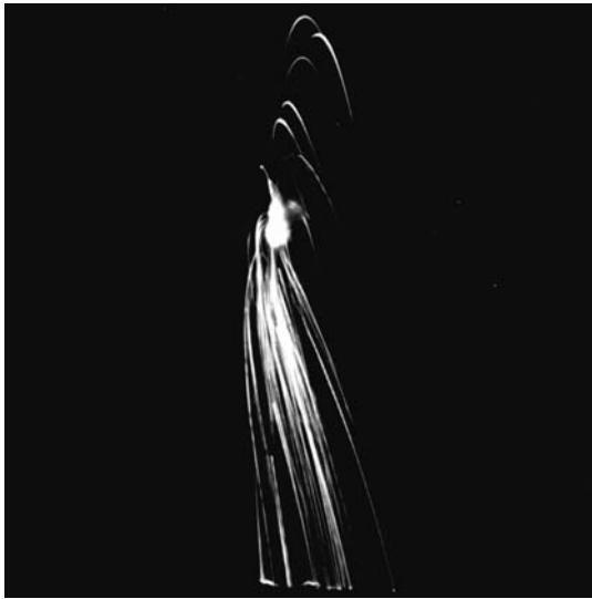
Photo 2. Ignition test, 10–20 mesh sponge.
