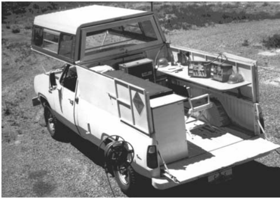
Photo 7. Mobile firing control center in bed of pick-up truck.
