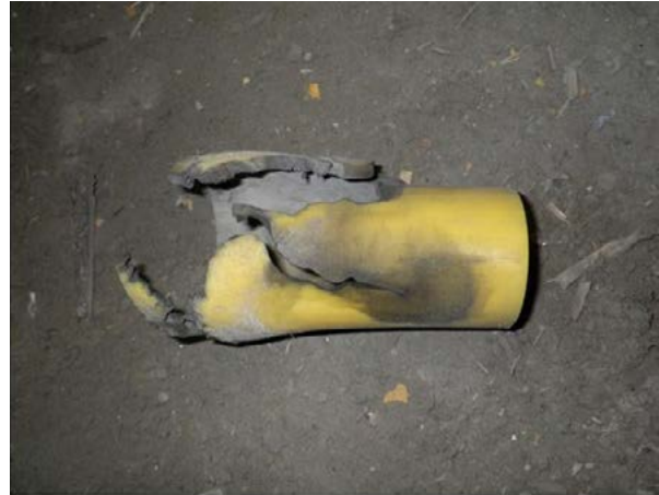
Figure 8. Ruptured plastic tube as a result of the second trial with the combination of squib 'HE 4' and the 'pear-shaped' NSP 711 charge.
