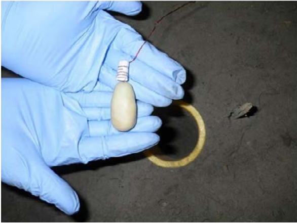
Figure 7. Setup of the 'pear-shaped' charge NSP 711.
