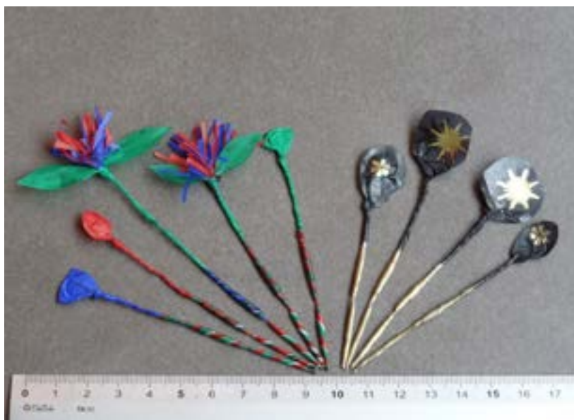
Figure 1. A collection of split-composition senko hanabi ‘Satori’ sparklers. The ‘Golden series’ sparklers on the right contain some sodium bicarbonate to generate a golden-yellow glitter finish. The nine depicted sparklers together weigh less than 1.5 gram.†
