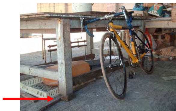
Plate 1. Wooden blocks used to level a working bench at a local fireworks factory. Source: author's own gallery.
