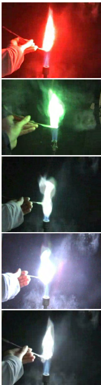
Figure 5. Color performance of (top to bottom) 5–9 in the flame of a Bunsen burner.
